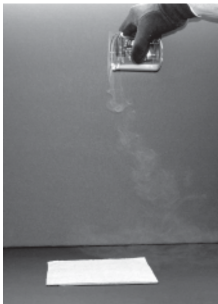
Figure 7. 1,1,1,2-tetrafluoroethane has a vapor density of 3.6 and falls rapidly but does not plummet as quickly as the trichloroethylene in Figure 6.
