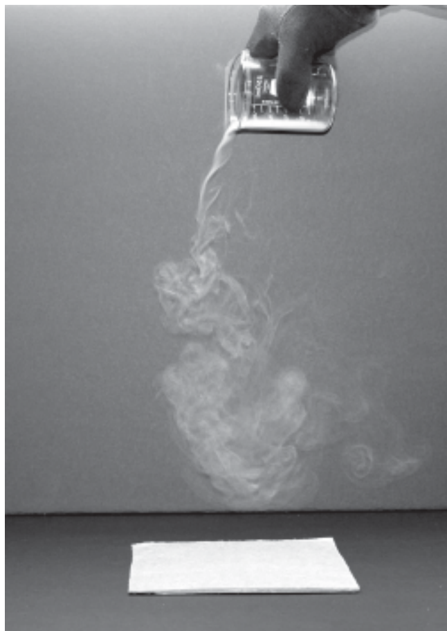
Figure 5. Tilt the beaker almost ninety degrees and observe the flow of the fume and vapor.
