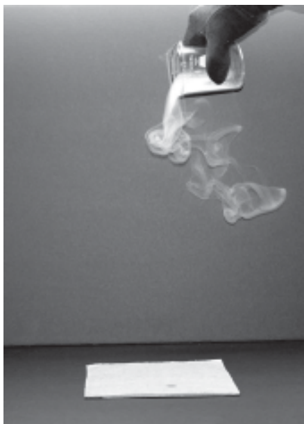
Figure 9. Isopropyl alcohol, 91%, contains water and produces a denser fume. The vapor density of isopropyl alcohol is 2.1 and the vapor density of moist air is less than dry air. This test measures the net buoyancy of the sample vapor and fume in air. Compare to hexane image with a lesser water content in Figure 9.
