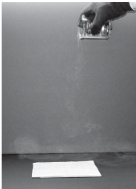
Figure 6. Trichloroethylene vapor (vapor density 4.5) remains in the beaker when the lid is removed and falls rapidly when the beaker is tipped.
