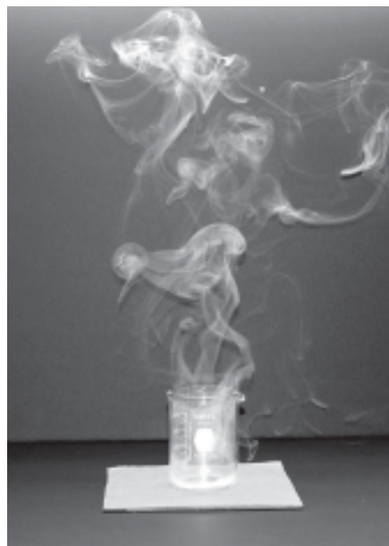
Figure 11. Ammonium hydroxide vapor and air current tube fume rise immediately upon removal of the lid. Ammonia has a vapor density 0.6 but dissolves into water vapor that also has a lighter-than-air vapor density.
