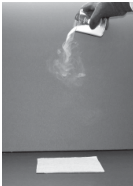
Figure 10. Starter fluid is a mixture of carbon dioxide (vapor density 1.53), ethyl ether (vapor density 2.6) and heptane (vapor density 3.5). The material safety data sheet for this product describes the vapor density only as "heavier than air." This test can be used to determine relative vapor density of mixtures in air.
